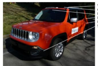
V2X antenna GNSS antenna Front RaCam Electronic Horizon Rear blind-spot Radar Side Ultrasound
